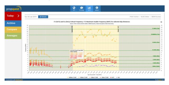
The valuable data that this site provides is the readings every 15 minutes for the frequency for Fof2 (aka Critical frequency) and the MUF (maximum usable frequency) for 100, 500, 1000
