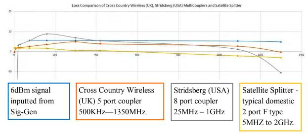
The graphed results are shown above. On the left is the dB in steps of 10 starting at the bottom with
